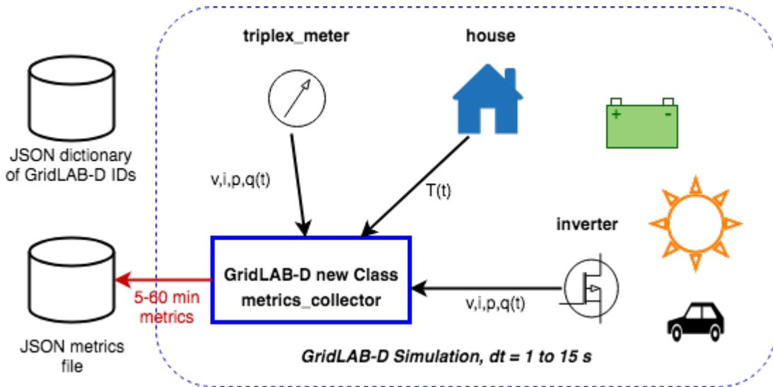
Fig. 5.8: New metrics collection classes for GridLAB-D
