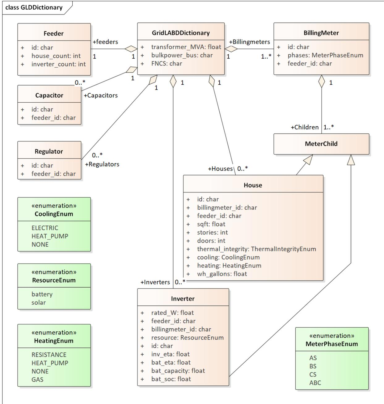
Fig. 5.10: GridLAB-D dictionary
