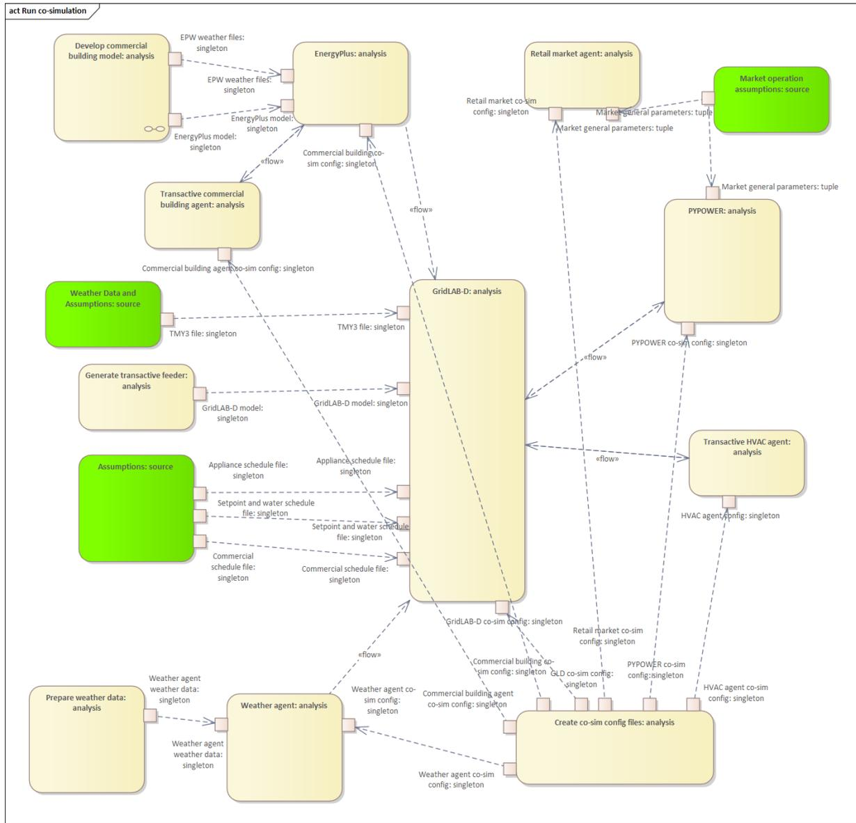
Fig. 3.18: Detailed model of the co-simulation process showing the dynamic data exchanges with “<<flow>>” arrows.
