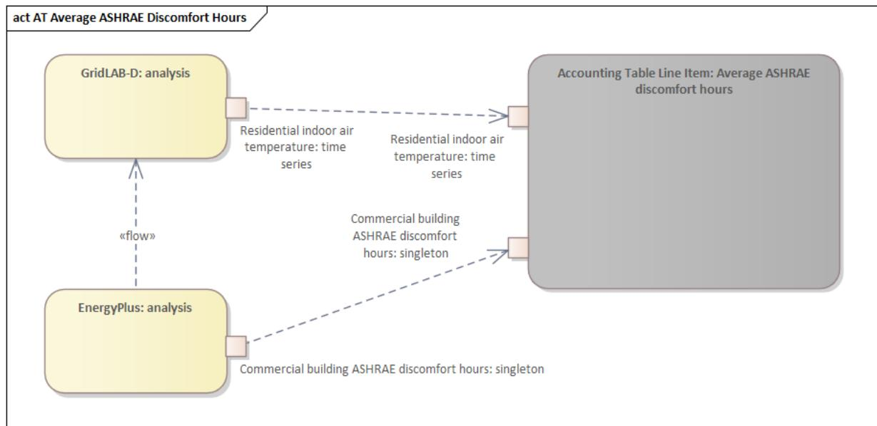
Fig. 3.19: Average ASHRAE discomfort hours metric data flow
