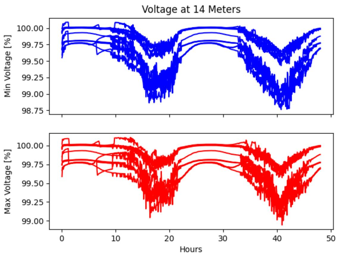
Fig. 3.6: Meter measurements of all houses in GridLAB-D
