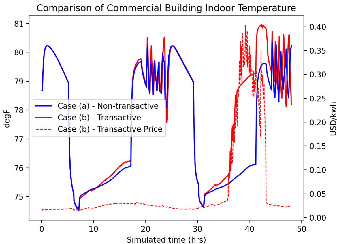
Fig. 3.44: Commercial building (as modeled in Energy+) indoor air temperature for the base and transactive case. Results should be similar to the residential indoor air temperature with lower temperatures during low-price periods and higher temperatures during high-price periods.
