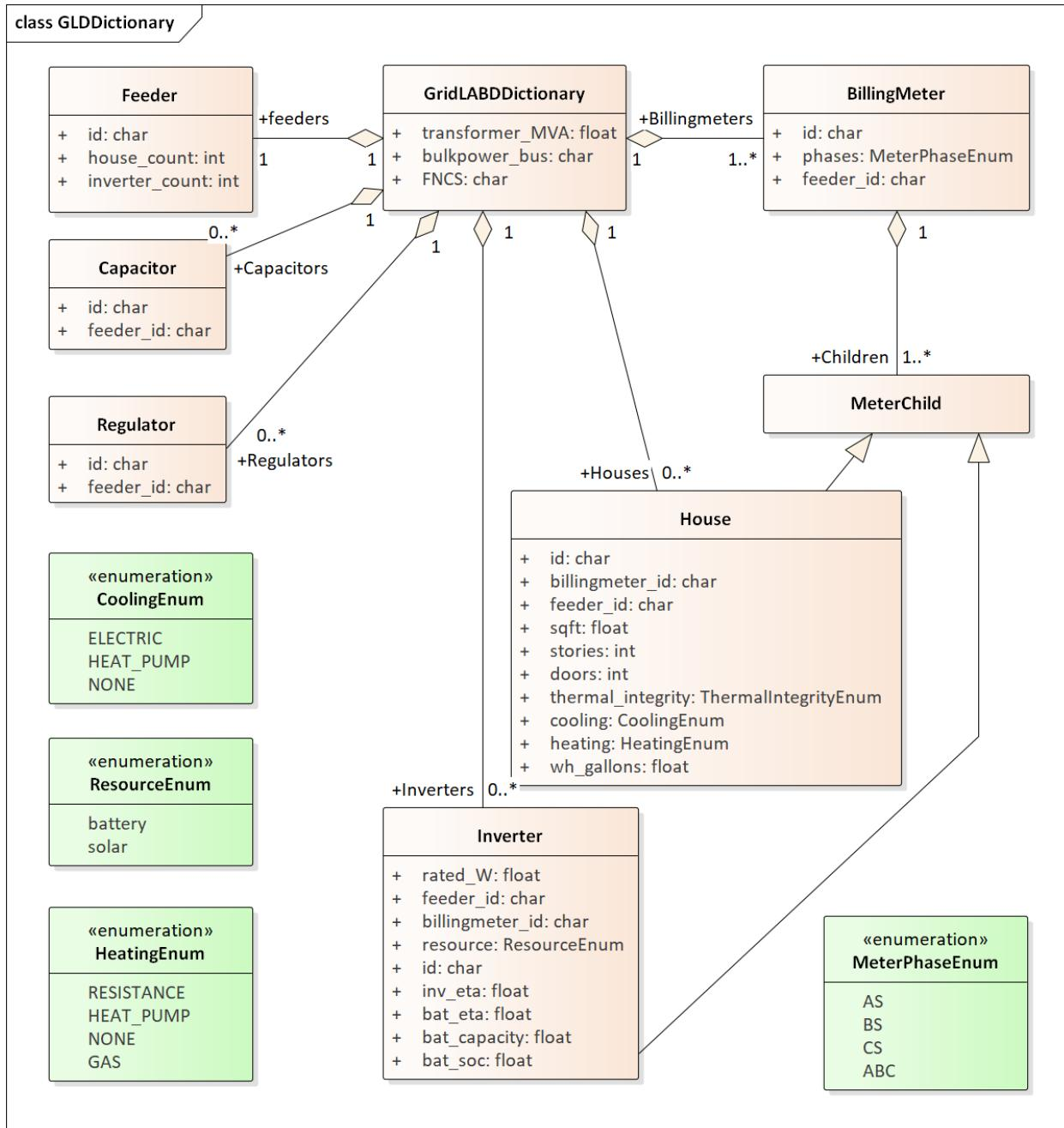
Fig. 5.10: GridLAB-D dictionary
