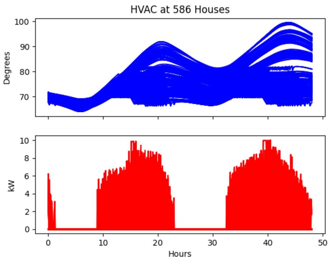
Fig. 3.5: Operation of all HVACs in GridLAB-D
