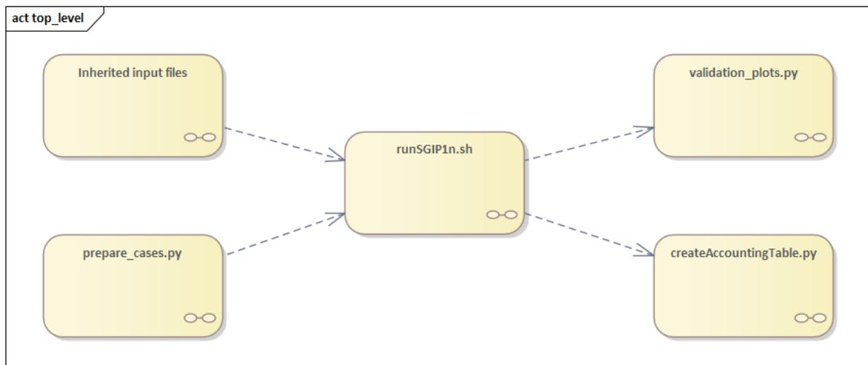
Fig. 3.33: Overview of the software execution path
