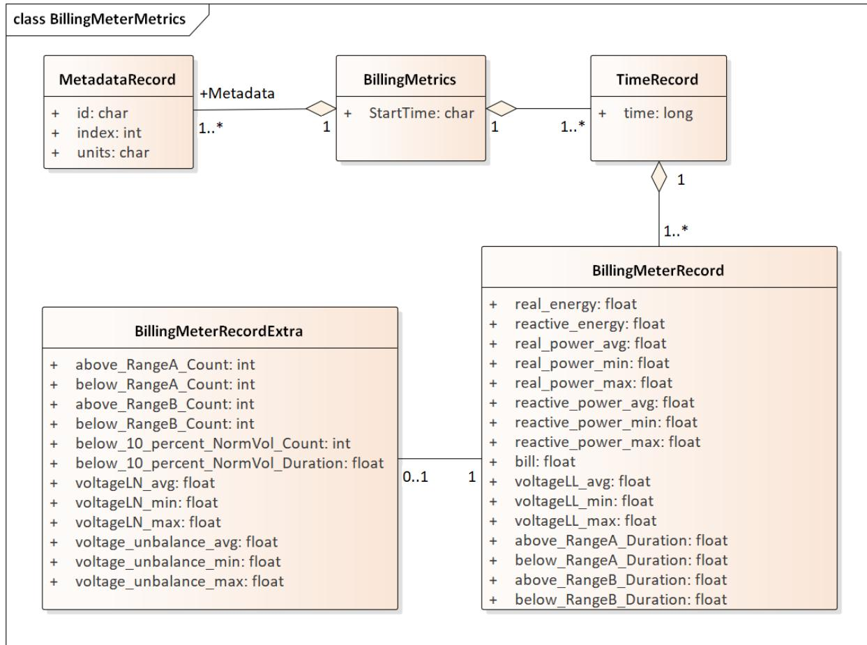
Fig. 5.14: GridLAB-D billing meter metrics
