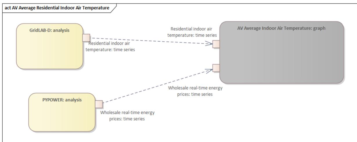
Fig. 3.25: Residential indoor air temperature metric data flows
