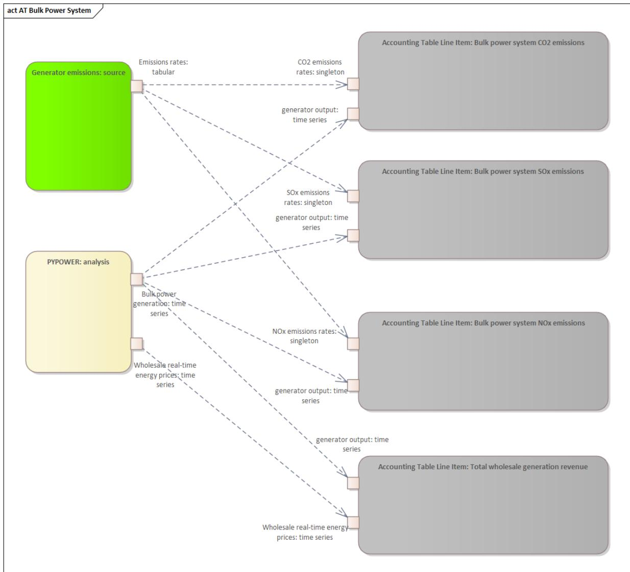
Fig. 3.20: Bulk power system (T+G) metrics data flows
