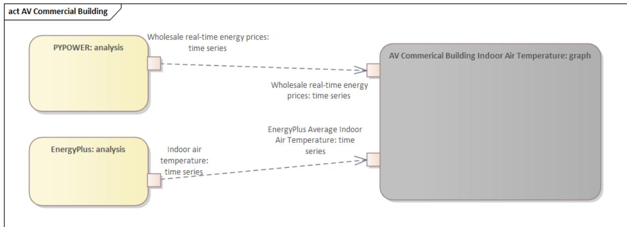
Fig. 3.26: Commercial indoor air temperature metric data flows
