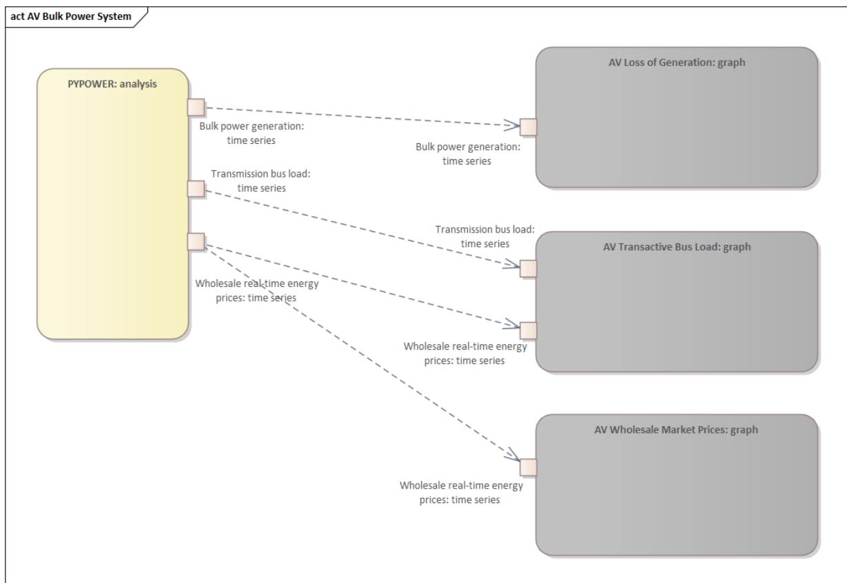
Fig. 3.24: Bulk power system metrics data flows
